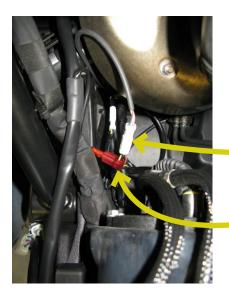
5. Locate the GPS (Gear Position Sensor) connector (small white three pin connector) near the bottom of the tank, behind the rear exhaust. Trim the wire sheathing back and crimp a supplied scotchlok onto the **yellow/green** wire of the factory GPS connector. Now insert the Bazzaz GPS connector (red connector with pink wire) into the scotchlok.
