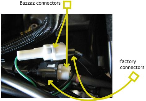
9. Locate Throttle Position Sensor (TPS) between airbox and frame on right side and disconnect the factory harness connector. Install corresponding Bazzaz connectors in line with factory harness; route harness between airbox and frame.
