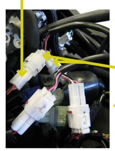
5. Locate speed sensor connectors (middle of engine compartment in rubber boot with other connectors) and install corresponding Bazzaz connectors inline with factory harness.
