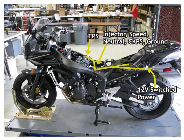
3. Route the Bazzaz +12V switched lead back towards the taillight following the factory harness on the left side of the bike. Pull back the harness sheathing to expose the wires of the factory harness of the tail light connector and crimp a supplied scotch lok connector onto the **blue wire**. Insert the Bazzaz +12V switched power connector (**red wire**) (orange tag) into the scotchlok.
