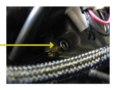
8. Locate Crank Position Sensor (CKPS) connectors (right side, just behind airbox) and install corresponding Bazzaz connectors inline with factory harness.
