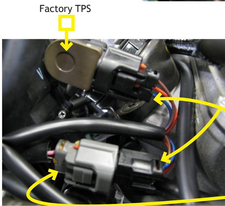
5. Locate the factory Throttle Position Sensor (**TPS**), which will be found on the rear throttle body (left side). Disconnect the factory TPS connector from the sensor and install the Bazzaz TPS connectors in-line with the factory connector and sensor.
