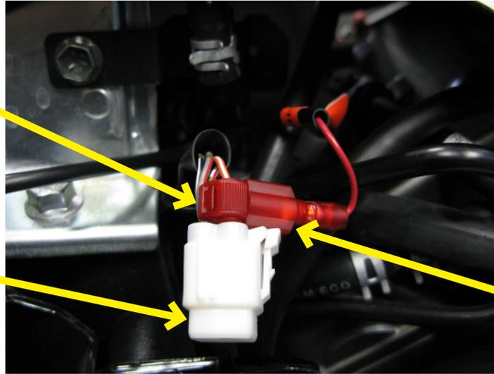
7. Locate the factory two-pin Crank Position Sensor (CKPS) connectors, which can be found on the right side of the bike along the frame. Once located, begin to route the Bazzaz CKPS lead between the rear throttle body and the rear valve cover. Disconnect the factory CKPS connectors and connect the Bazzaz CKPS connectors in-line with the factory connectors.
