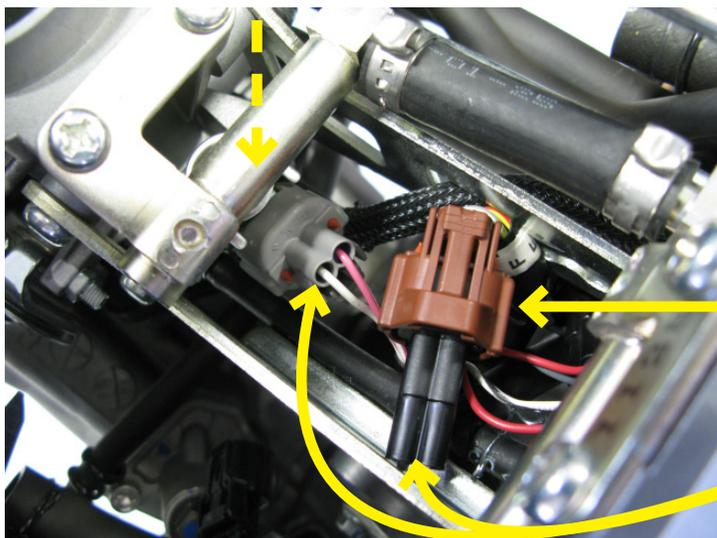
9. Now disconnect the **INJECTOR # 2** (rear cylinder injector) factory connector from the injector and install the Bazzaz injector # 2 connectors in-line with the factory injector and connector.
