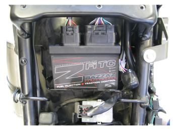
3. Connect the main connector of the Bazzaz **FUEL HARNESS** to the control unit. Begin routing the harness towards the engine compartment and down the left side.
