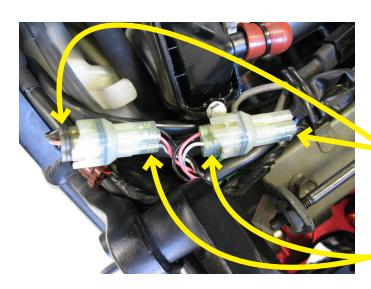
5. Next, locate the factory Gear Position Sensor (GPS) connectors, which can be found near the factory fuel pump connector. Disconnect the factory GPS connectors and connect the Bazzaz **GPS** connectors in-line with the factory connectors.
