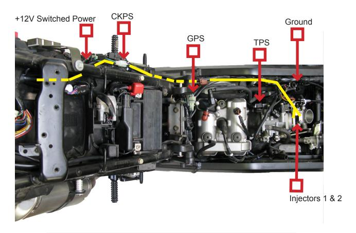
Harness routing shown in yellow. Stock component identification and location shown for reference.
