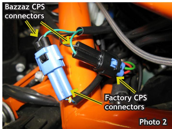
3. Continue to route this portion of the harness toward the rear of the air box inside the frame. Locate the factory gear position sensor connectors found between the frame and rear cylinder (photos 3 & 4). Disconnect the factory connectors and install the mating Bazzaz Gear Position & Neutral connectors in line.
