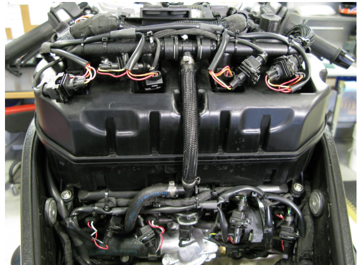
Bazzaz harness installed in-line with both lower and upper injectors. Note: The routing of the Bazzaz harness in relation to the injectors flows from left to right on the motorcycle.
