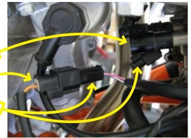
7. Next, locate the factory diagnostic connectors which can be found towards the front of the airbox. Disconnect the factory diagnostic connectors and install the Bazzaz **+12V SWITCHED POWER** connectors in-line with the factory connectors.
