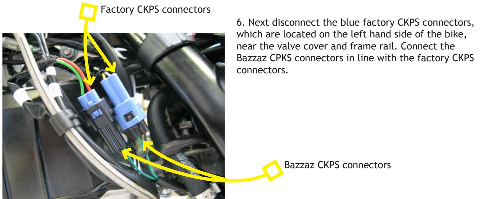
6. Next disconnect the blue factory CKPS connectors, which are located on the left hand side of the bike, near the valve cover and frame rail. Connect the Bazzaz CKPS connectors in line with the factory CKPS connectors.
