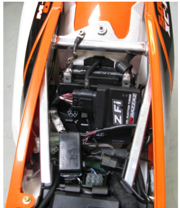
3. Connect the Bazzaz fuel harness to the control unit. Begin routing the harness forward, towards the engine on the left hand side, between the air box and the sub frame. Locate the factory diagnostic four pin, clear connectors on the right hand side of the bike (near the front of the battery). Disconnect the factory connectors and install the Bazzaz switched power & ground connectors in line with the factory connectors.
