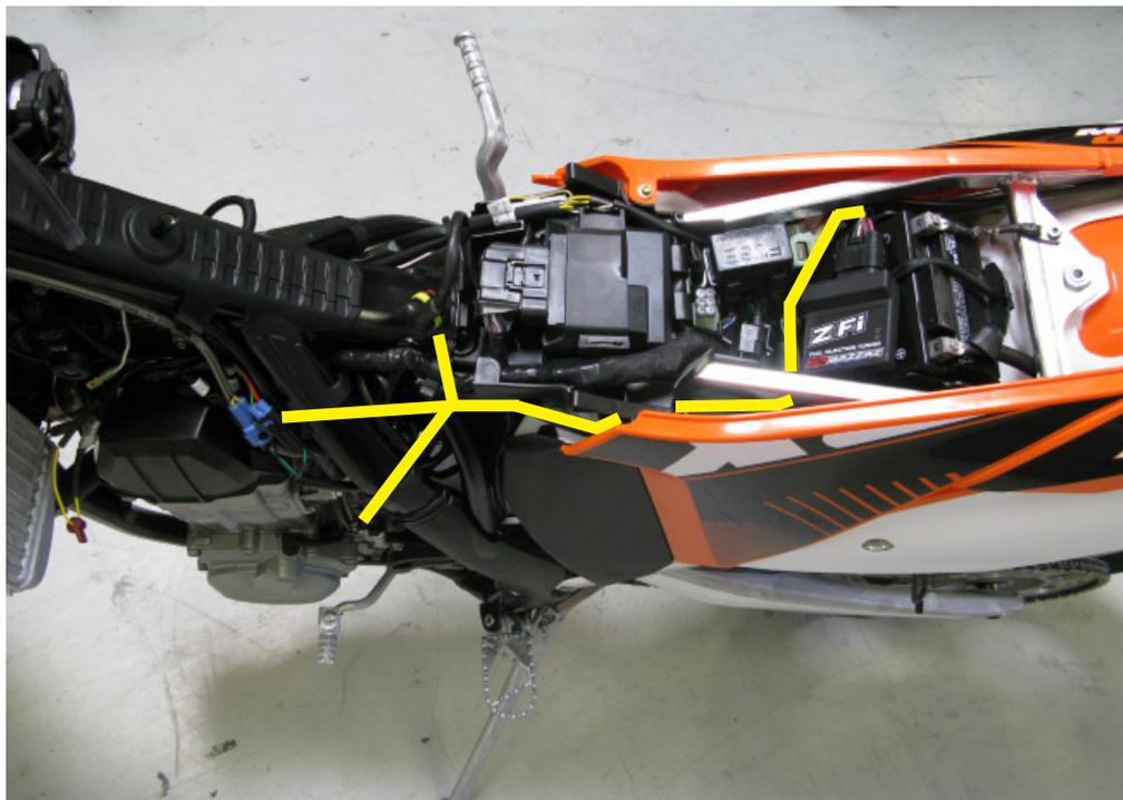
1. Begin the installation by removing the rider seat, radiator shrouds and tank.
