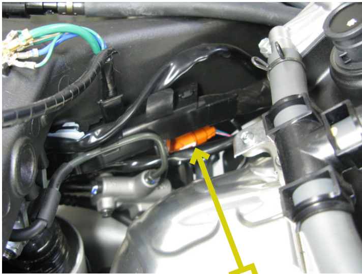
factory rear wheel speed sensor
