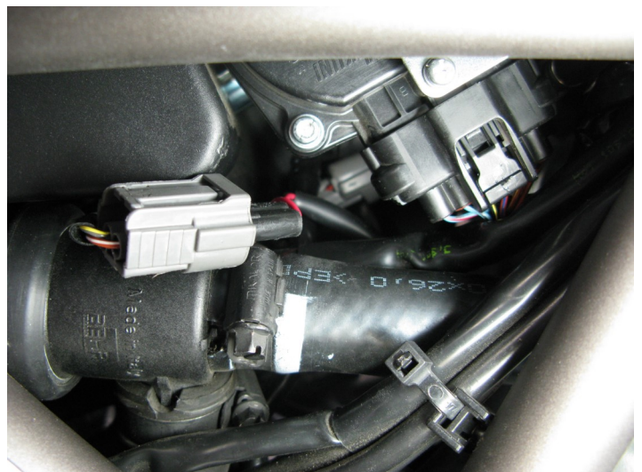
Bazzaz harness installed in-line
