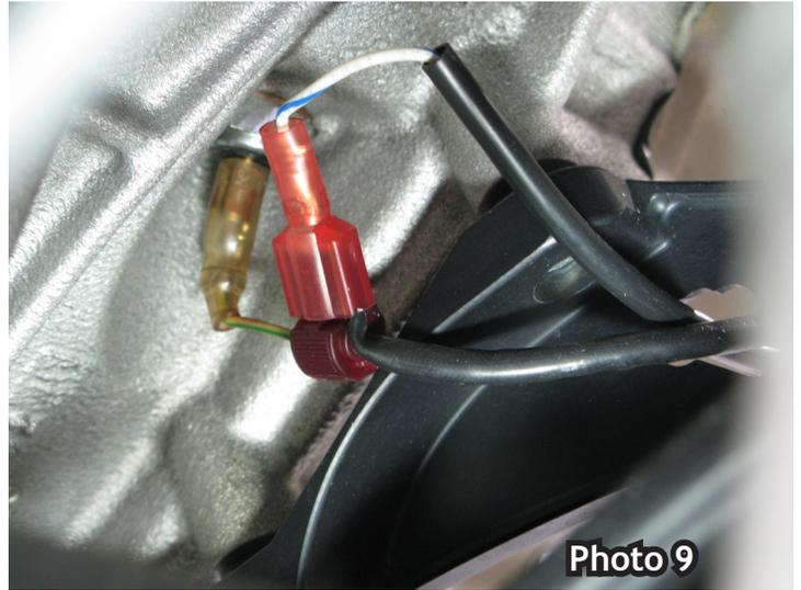
Route the remainder of the Bazzaz harness containing the throttle position, injector connectors and ground between the front and rear cylinders to the left side of the motorcycle.
