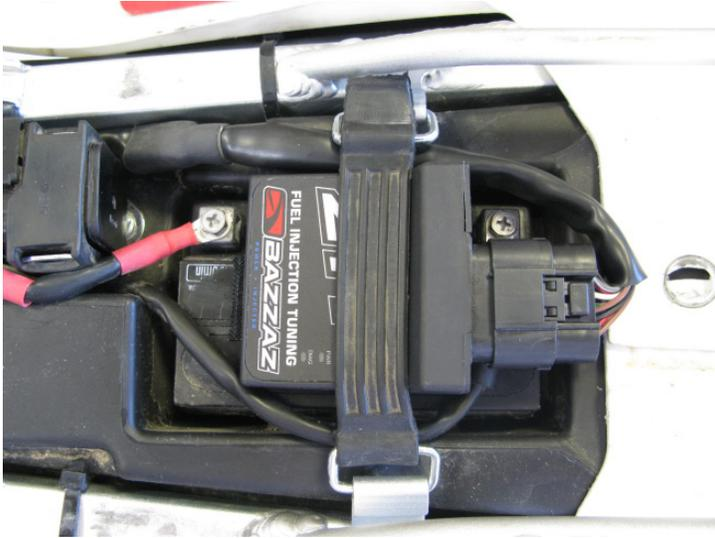
3. Connect the main connector of the Bazzaz fuel harness to the control unit and begin routing the harness (highlighted in yellow) back toward the engine on the right hand side.
