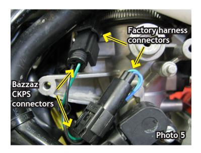
8. Disconnect the factory harness throttle position sensor connectors from the sensor and install the mating Bazzaz harness connectors inline (photo 6).
