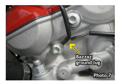
10. Now that the installation is complete, take a moment to secure the Bazzaz harness along its routing path with the supplied cable ties. Reinstall the components removed in step one of these instructions.
