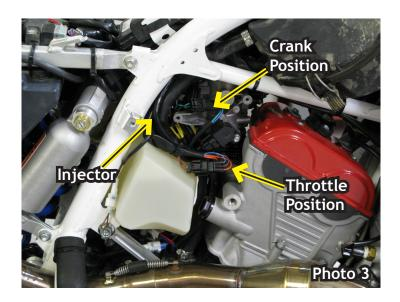
6. Identify the injector connector which can be found at the rear of the throttle body assembly under the factory ECU. Disconnect the factory harness connector and install the mating Bazzaz harness injector connectors inline (photo 4).
