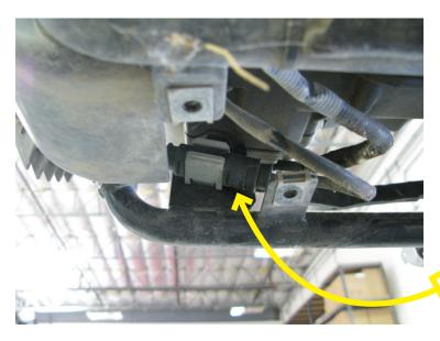
8. Now you will need to eliminate the factory **O2/ LAMBDA SENSOR**, as this sensor will no longer be used. The sensor connector is a round four-pin connector, found attached to the right side of the frame and under the skid plate. Simply disconnect the connectors; the wires should be neatly secured away from any moving components, or the sensor may be removed and the remaining port/bung in the exhaust can then be plugged.
