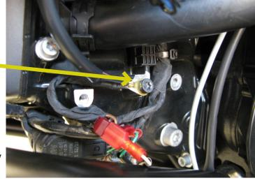
insert the Bazzaz GPS connector (red connector with pink wire) into the scotchlok.
